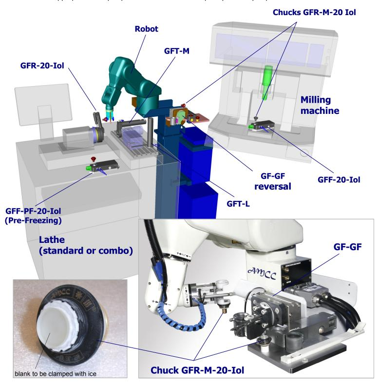
These units work in association with traditional **AMCC** freezing devices, and combo or traditional lathe and milling machines from worldwide manufacturers.
