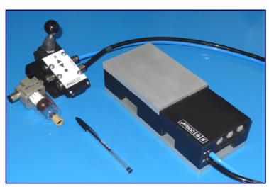
part to be machined. Turn then the pneumatic valve lever on "ice" position. Within seconds the water freezes and the part is clamped. Unclamping, just as fast, is done by moving lever to "thaw" position.
