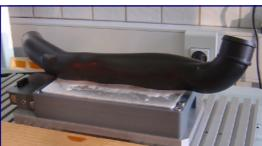
Fitting a supporting plate between the part and the plate produces a sandwich bound by ice. Since the milling tool emerges full into the material, the part to be machined can be trimmed with no excess vibration or profile chipping.
