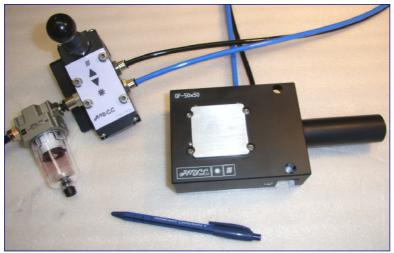
Connect the filter to the compressed air system<sup>3</sup>, spray water onto the icing plate and position the part to be machined. Turn then the pneumatic valve lever on "ice" position. Within seconds the water freezes and the part is clamped. Unclamping, just as fast, is done by moving lever to "thaw" position.
